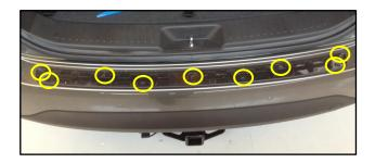
2. Use a plastic removal tool to carefully lift the corner of the bumper protector base.
