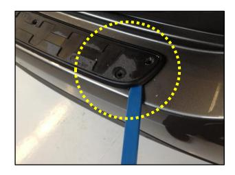
3. Remove bumper protector base by pulling upwards.
