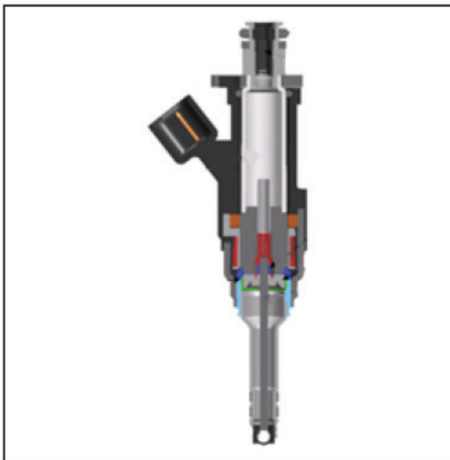
The internals of the Injector are designed to minimize the formation of deposits
