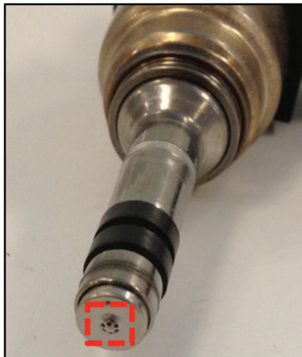
New injector showing location of Spray Orifices
