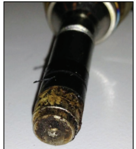
Normal injector appearance while in service
