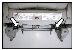
2. Check the current position for the seat release cable adjuster. The default setting from the factory is in slot two (2).
