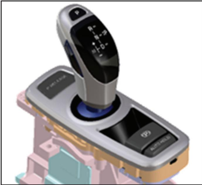
The Shift by Wire or SBW system is all new in select Kia K900 models for 2015. Paired with the 8 speed transmission, this advanced electronic shifter provides for easier gear selection and customer convenience. Faster shifting with less movement enhances an independent gear shift pattern with a different gear selection order than conventional shifters.
