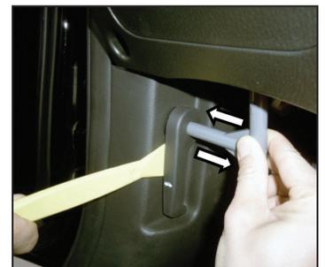
2. While applying slight inward pressure to the end of the SST, use a plastic prying tool to remove the hood release lever.
