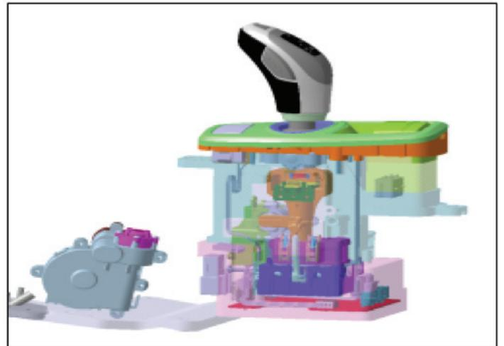
If vehicle wheel rotation is detected the cable actuator is energized pulling the cable and keeping the parking pawl from engaging.
