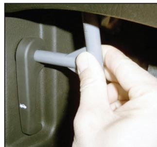
1. Insert the SST into the hole on the hood release lever, as shown.
