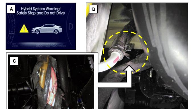
NOTE: If the "Hybrid System Warning!" message appears in the cluster without a DTC present in the system, call Techline for further assistance with diagnosis.
