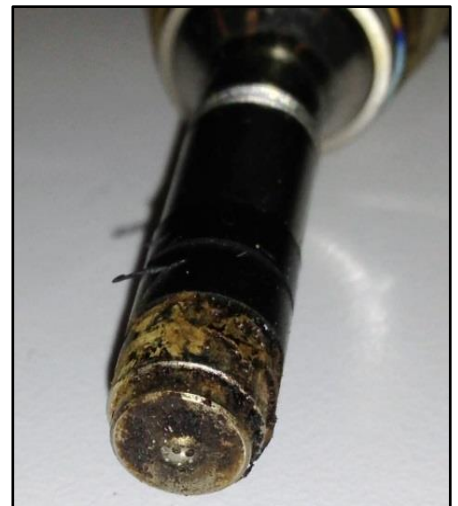
Normal injector appearance while in service
