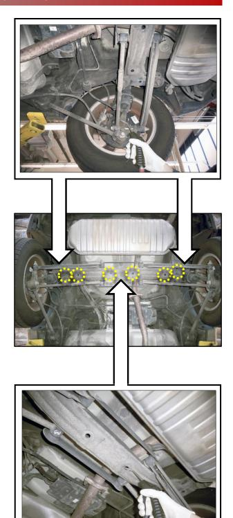
8. Remove any debris from the inside of the cross member using an air gun. Make sure to insert the nozzle in multiple holes and rotate it in all directions to completely remove any foreign material or rust flakes.
