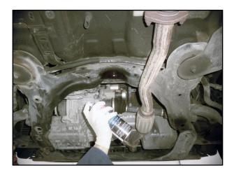
6. Apply undercoating onto each rear lower control arm and trailing arm. Avoid overspraying other parts of the vehicle.
