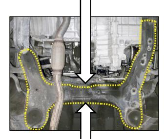
4. Remove any debris from the inside of the sub-frame using an air gun. Make sure to insert the nozzle in multiple holes and rotate it in all directions to completely remove any foreign material or rust flakes.
