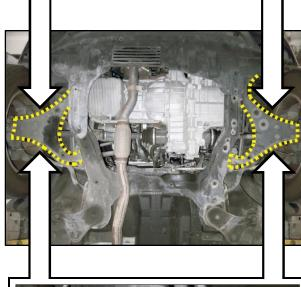
Remove any debris from the inside of each front lower control arm using an air gun. Make sure to insert the nozzle in multiple holes and rotate it in all directions to completely remove any foreign material or rust flakes.
