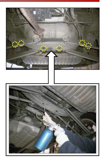
4. Apply undercoating onto the upper and lower surfaces of each front lower control arm. Avoid over-spraying other parts of the vehicle.
