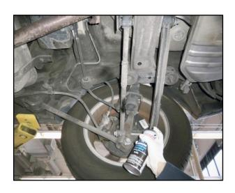
7. Apply undercoating onto the upper and lower surfaces of the cross member, as shown. Do <u>NOT</u> apply undercoating to the exhaust pipe or other unrelated parts of the vehicle.
