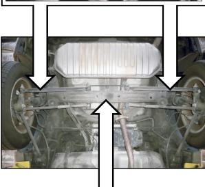
6. Use a metal bristle brush to clean and remove any rust scales or contaminants from all surfaces of the <u>rear cross member</u>.
