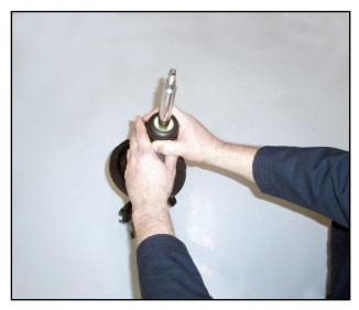
6. Pull the dust cover and bump stop until the bottom lip of the dust cover is slightly below the strut body.
