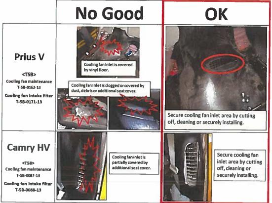
Caution: Failure to cut out vinyl cover at HV Battery cooling system air inlet screen area will result in premature HV Battery damage
