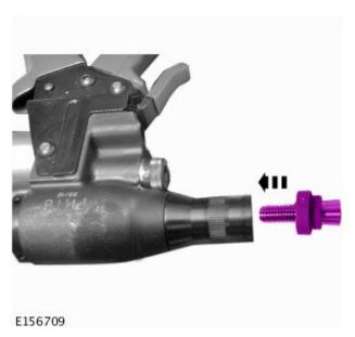
ONOTE: The earth stud bond is totally selfsealing and watertight; there is no need to dress the hole with any primer before fitting.
