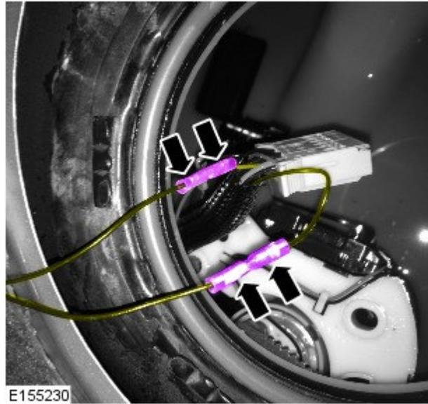
22. Measure the resistance values of the fuel gauge sending units.
