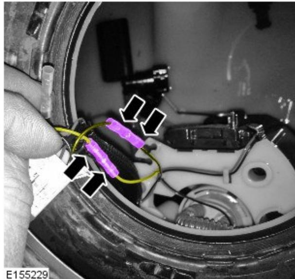
21. **⚠ CAUTION: After crimping the connection, perform a gentle pull test to make sure that a sufficiently strong connection has been created. If required, remove and replace the splice.**
