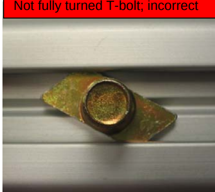
Not fully turned T-bolt; incorrect
