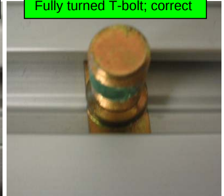
Fully turned T-bolt; correct
