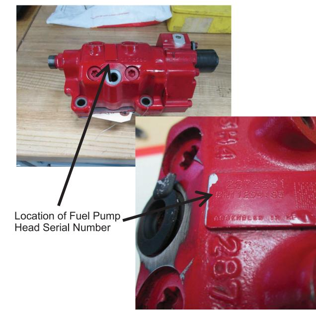
Mark the Fuel Pump Head part number with a paint marker after completing the campaign.
