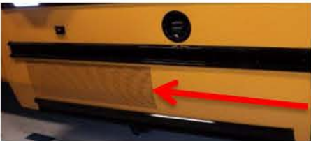
Fuel Fill Hose under bus behind driver's side skirt
