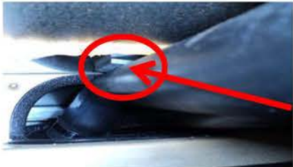
Seat mount plate sharp edge could rub on the fuel fill
