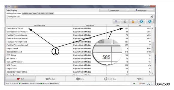
The fuel pressure value displayed on the Data Display screen is 585 kPa (85 psi). This is an example of a good fuel pressure reading. Do NOT replace the fuel pump module if the fuel pressure readings are equal to or above 500 kPa (73 psi).
