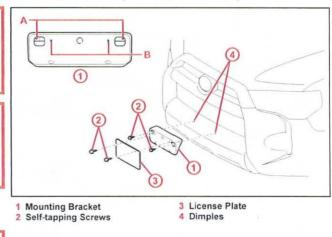
NOTICE Do NOT overtighten the self-tapping screws.
