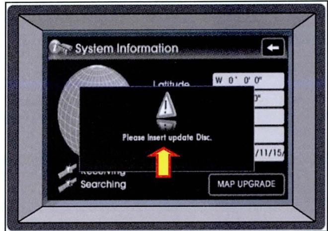
5. Insert the Orange disc, and wait for it to read the contents. Press the **“Yes”** button to continue with the software update process.
