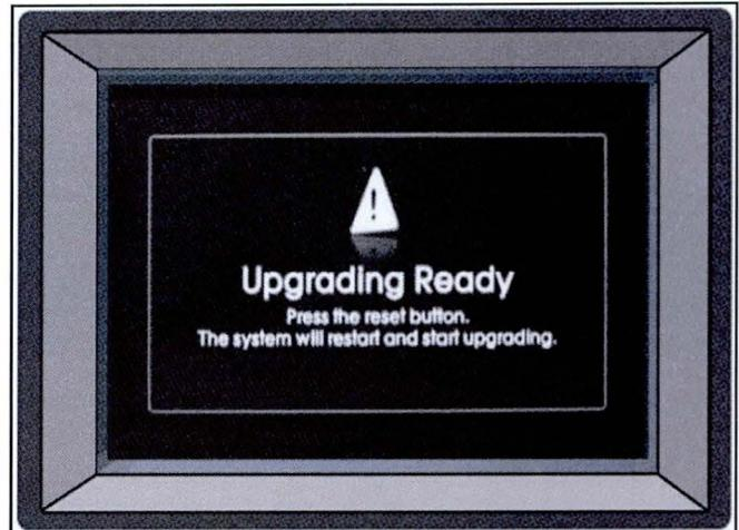
Press and hold the **Reset Button** for 3 seconds using a pen or paper clip and then release.
