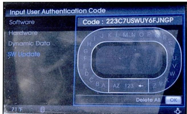
**3.11** The authentication code should be entered on the screen as shown to the right, using the CCP (Center Control Panel), and then select 'OK'.
