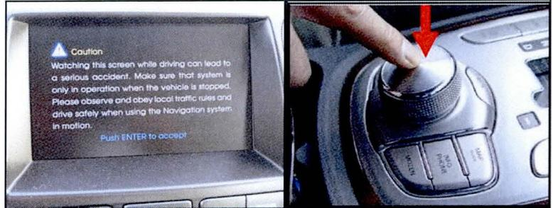
3.20 Enter the software update menu by **simultaneously** pressing the [B] DISC/AUX, [C] BACK, [D]NAVI/MENU buttons while pressing the [A] VOL KNOB.
