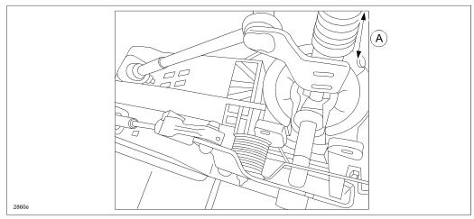
9. Check that the cable adjustment condition (number of thread turns (A)) has changed from the previous check.
