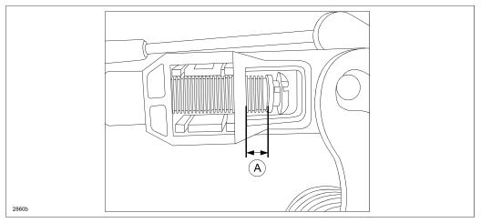
6. Release the safety lock (A) by sliding it to the direction of the arrow shown.
