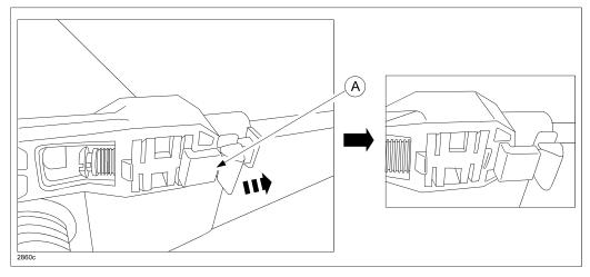
7. Release the locking piece (A) by pushing it from the back.
