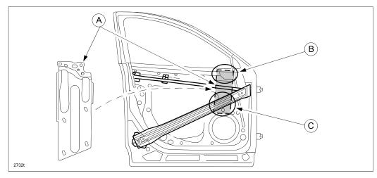
While holding the power door mirror, temporarily place the reinforcement with the three (3) power door mirror bolts through the holes in the reinforcement, then tighten the bolts.
