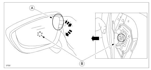
Move the mirror glass left and right and up and down to make a space for your fingers to insert in the back of mirror glass. Press the mirror glass with your fingers toward you to disconnect the joint for adjustment gears (A) and (B).
