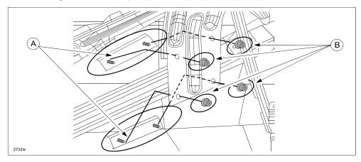
13. Tighten the four (4) nuts (B) to secure the reinforcement onto the side impact bar-lower. Tightening Torque: 15 ft. lbf. {2.1 kgf-m, 20 Nm}
