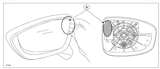
4. Press the black plastic base at the back of mirror glass (A) toward you and carefully disconnect the joint with the center pivot (B).
