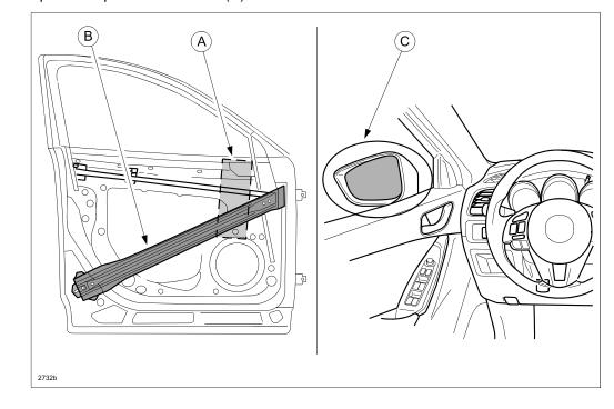
**Repair B:** Replace the power door mirror (C) with a modified one.
