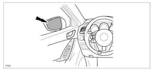
This concern may be due to a lack of rigidity of the mirror base so the mirror vibrates when it receives vehicle vibration or wind pressure.
