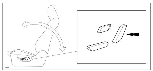
The configuration of the recliner switch knob has been changed to eliminate this concern.
