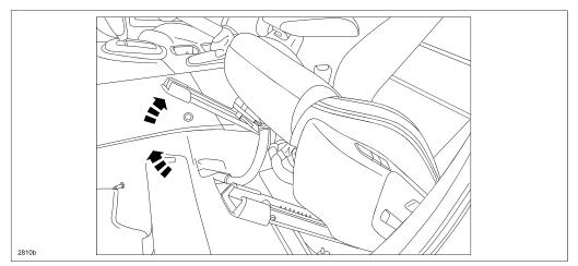
7. Insert an appropriate tool between the frame and the cable (the general area is shown below/left). Use the tool as a lever to release the cable from the center bracket (50mm from the motor as shown below/right).
