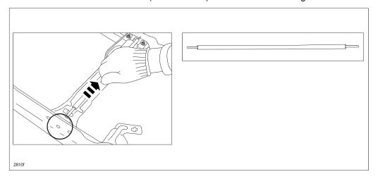
11. Align the square tip of the new cable to the square shape in the motor. Push the cable all the way in (A) using care not to damage or deform it.
