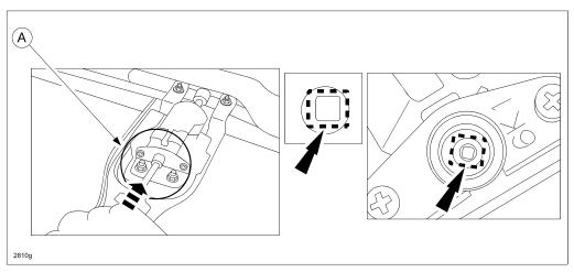
12. Align the square tip of the cable to the square shape in the gear box. Push the cable all the way in.
