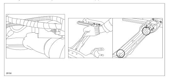
9. Pull the cable in the direction of the arrow (as shown below) to remove it from the motor.
