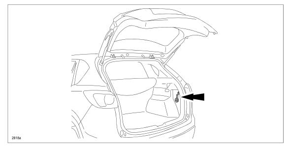
An EPT sealer has been attached to the theft deterrent horn during mass-production to eliminate the noise. Customers having this concern should have their vehicle repaired using the following repair procedure.
