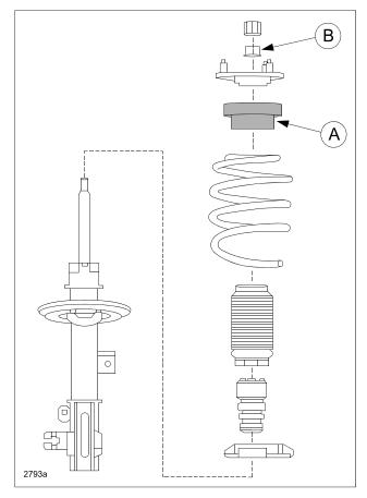
The noise may be due to the upper housing of the front strut bearing being damaged when applying excessive force to the bearing during customer use. To eliminate the noise, the material and production method of the front strut bearing has been changed.
