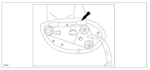
5. Using pliers, snap off the boss where the push nut (A) is installed, then remove it (B).
