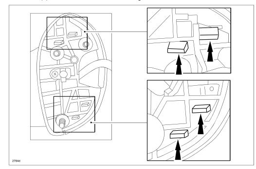
6. Disconnect the four (4) connections shown below using a flathead screw driver.
