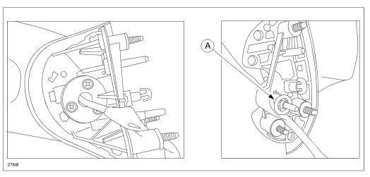
14. Align both locators (A) and install the base cover to the inner base as shown below.
