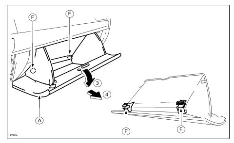
d. Pull the glove compartment (A) in the direction of the arrow (4) and remove it while detaching hooks (F).
