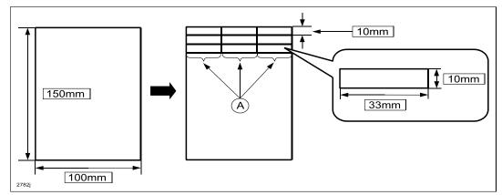
11. Stack three of the 10 X 33 mm non-woven fabric pieces together (total of 0.75mm thickness).
