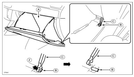
c. Pull down the glove compartment (A) in the direction of the arrow (3).
