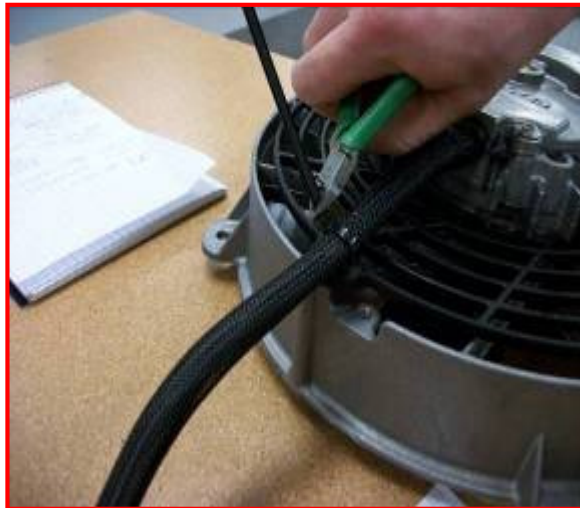
Figure 15: Securing and Trim of Zip Tie
