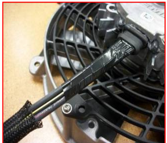
Figure 10: Fan Harness Taped
