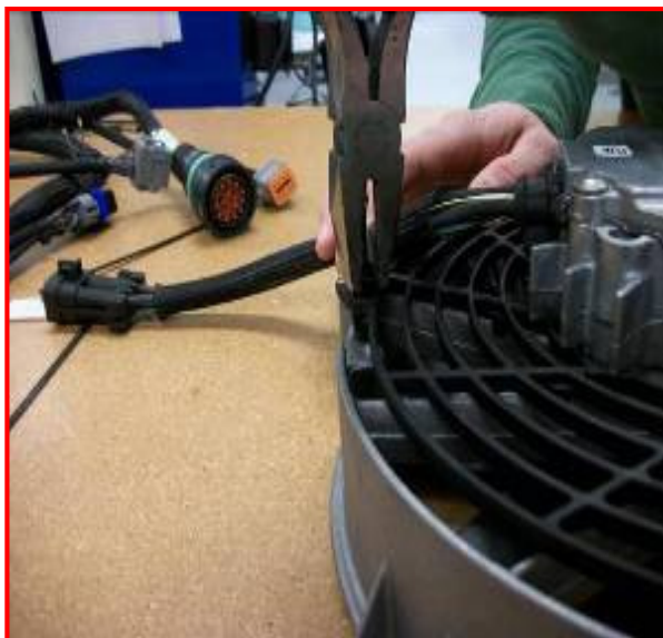
Figure 6: Removal of Zip Tie (2)
