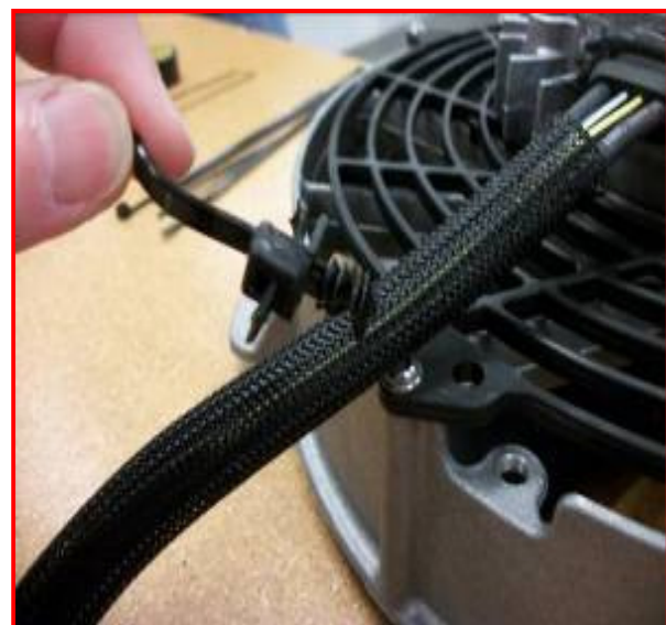
Figure 7: Zip Tie Removed
