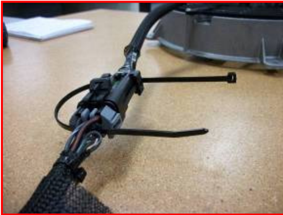
Figure 25: Zip Tie Inserted
