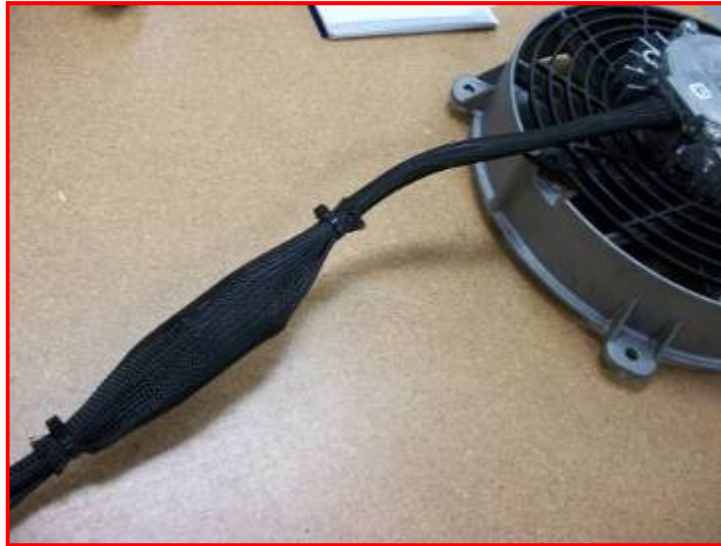
Figure 33: Protective Sleeve for Fan Connection
