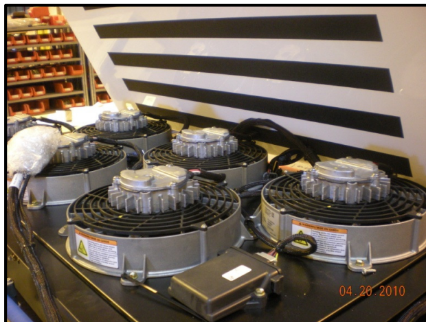
Figure 1: Rooftop Oil Cooler
