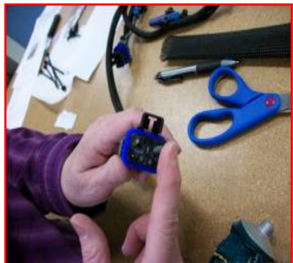
Figure 20: Smear Grease Over all Pins
