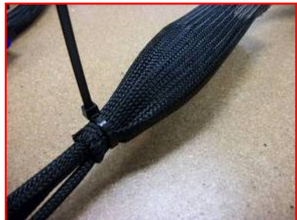
Figure 28: Zip Tie Protective Sleeve on Harness
