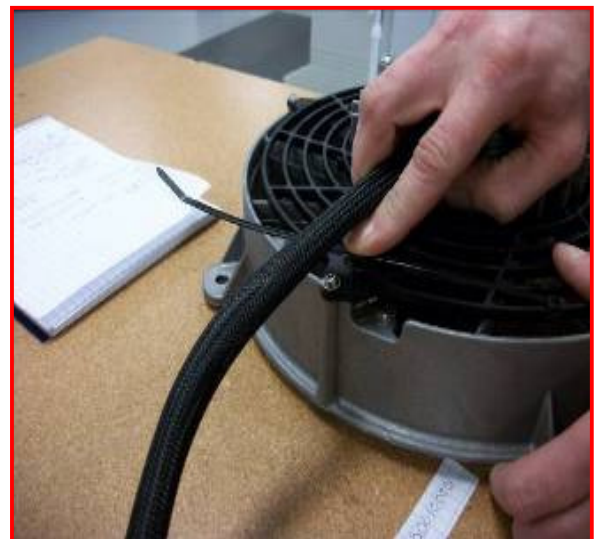
Figure 14: Installing Zip Tie into Guard
