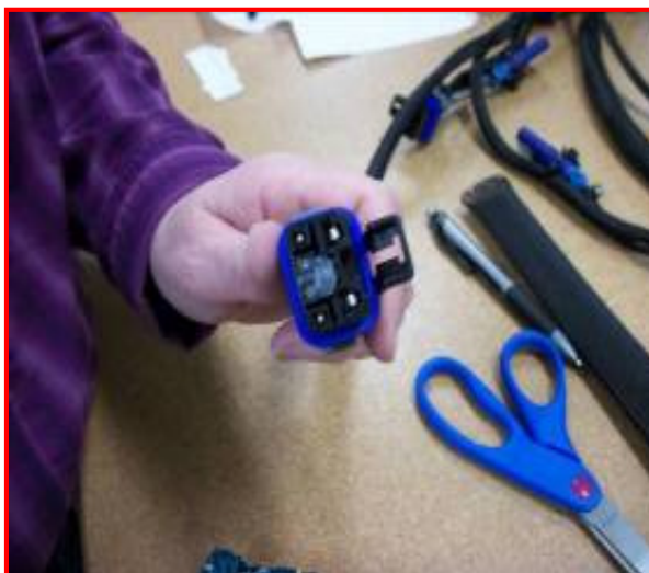
Figure 19: Di Electric Grease on Connector
