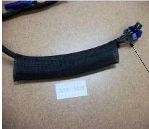
Figure 18: Braided Material Over Main Harness
