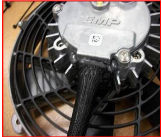
Figure 12: Sleeve Over Header
