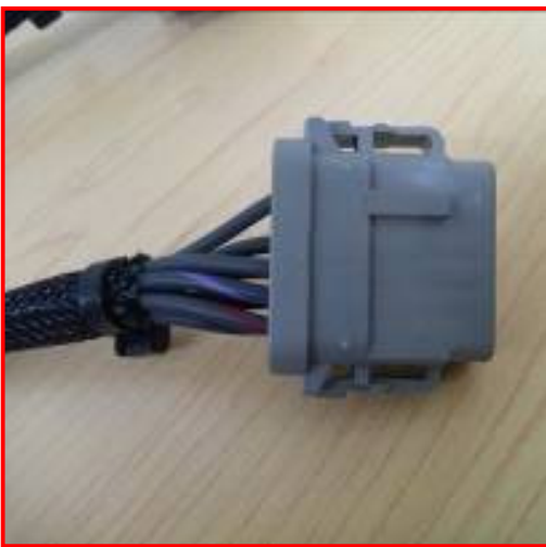
Figure 34: Wires exposed on TMC Connector
