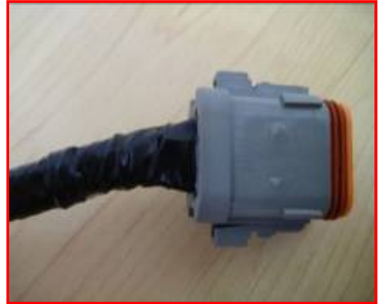
Figure 35: Wires taped on J1939 Connector
