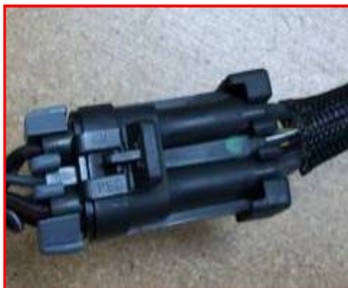
Figure 23: No Seal Visible, Correct
