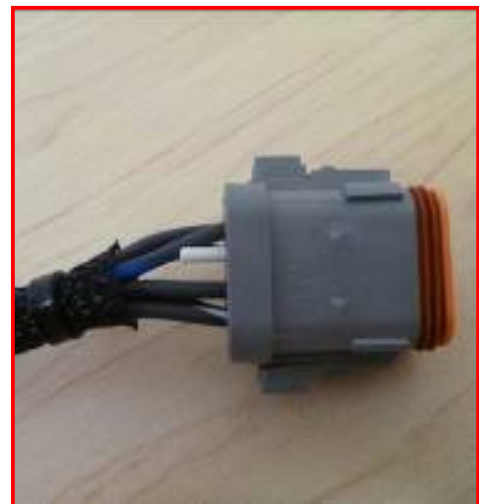
Figure 35: Wires exposed on J1939 Connector
