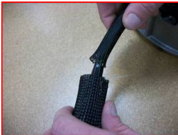
Figure 29: Braided Sleeve Before Extension
