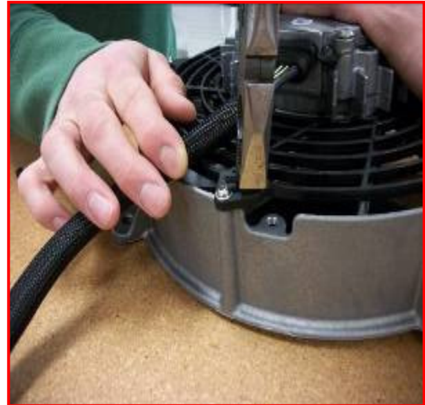
Figure 5: Removal of Zip Tie (1)
