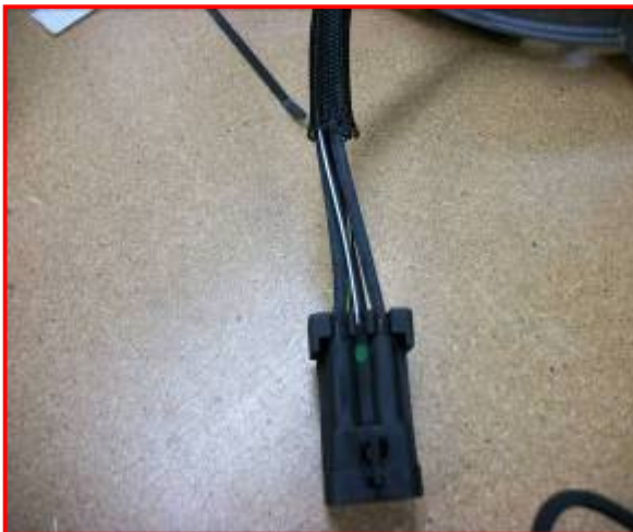
Figure 16: Exposed Wires on Fan Harness
