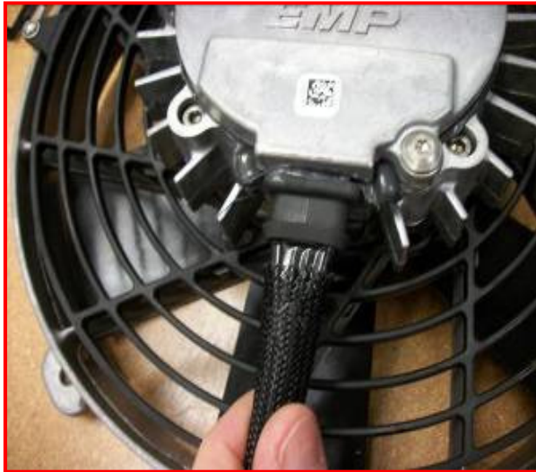
Figure 11: Sleeve Near Header
