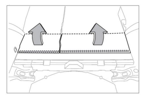
• If the vehicle <u>is not</u> equipped with Keyless Access / Push Start, the only repair is to install the revised rear floor spacer retaining clip as shown in the illustration below. Always use the proper trim clip removal tool to avoid damaging the clips and/or the spacer.
