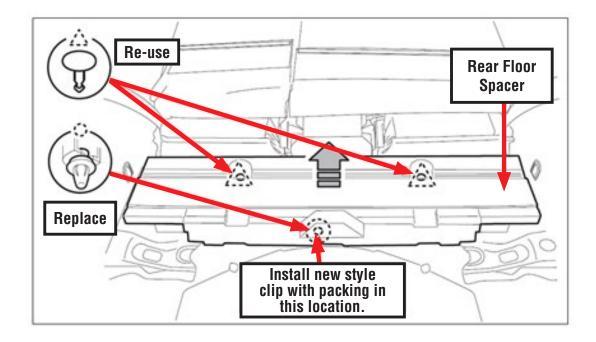
• If the vehicle **is equipped** with Keyless Access / Push Start, carefully remove the 3 retaining clips then the rear floor spacer to access the center antenna assembly. Replace the antenna assembly (which also includes a revised retaining clip) following the procedure in the applicable Service Manual. Torque the antenna bracket retaining bolt to 7.5 Nm (5.5 ft. lbs.). Make sure to use the new style retaining clip as shown in the illustration above when installing the floor spacer.
