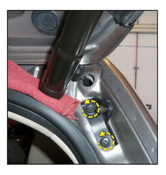
6. Replace the old bracket with the modified lifter mounting bracket. Make sure to apply upward pressure when tightening the retaining bolts to ensure bracket is as far up as possible.
