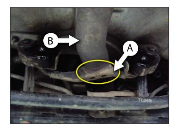
2. Check to determine whether the center muffler pipe hanger bracket (C) has become partially or completely separated from the muffler pipe (B).
