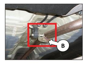
To correct this condition, without replacing the muffler pipe assembly, Kia is providing replacement bracket kits available as service parts. Follow the procedure in this bulletin to install a replacement bracket kit and correct the concern.
