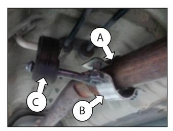
2. Install the rubber hanger (C) to the support on the vehicle and tighten the hanger bracket to the specification below.
