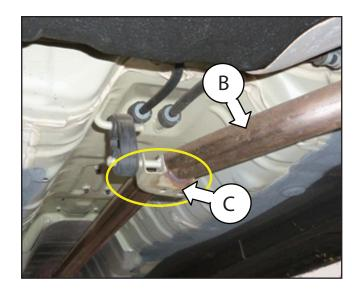
3. If either or both muffler pipe hanger brackets have *completely* separated from the muffler pipe, replace them with a new bracket, following the procedure on the next page. If either or both muffler pipe hanger brackets are only *partially* separated, use a grinder to separate them completely from the muffler pipe.
