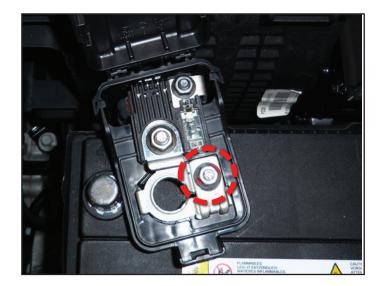
4. Use a flathead screwdriver to slightly spread open the terminal, as shown.
