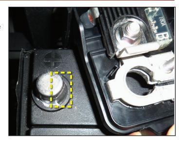
6. Re-install the battery terminal onto the positive battery post. Make sure the terminal is fully seated before installing the clamp and nut.
