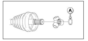
Carefully remove the trunnion assy. (B) from the driveshaft (A) using a suitable puller. Use a shop towel to remove any excess grease.
