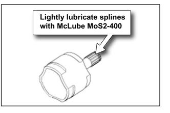
9. Replace all affected parts and reassemble the axle by reversing the order of removal. Be sure to follow exact instructions as outlined on KGIS information to prevent boot damage during reassembly
