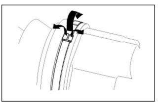
3. Carefully slide the boot along the driveshaft and away from the tripod joint. Clean excess grease from the assembly using a shop towel.
