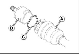
6. Using snap-ring pliers, or an equivalent tool, carefully remove the snap ring (A) from the driveshaft, as shown.
