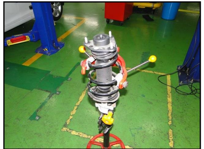
Press the coil spring downward (D).
