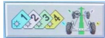
3. Continue to balance and tag all four assemblies. After all are completed, the screen will show tire positioning and the effect on tire pull or vibration. The purple horizontal arrow at the top of the screen shows overall pulling force and direction due to tires. The brown vertical arrows above each tire show the RFV of each assembly.
