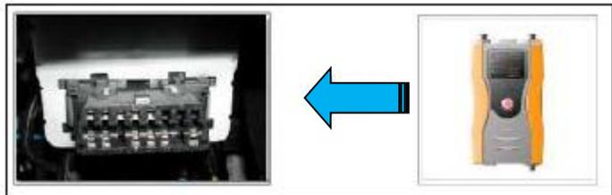
5. With the ignition key ON, turn ON the VCI and GDS tool. Access the GDS vehicle identification number (VIN) screen and configure the vehicle using the VIN AUTO DETECT Function.
