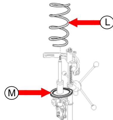
8. Assemble the new left front strut and all other removed strut related components in reverse order of disassembly.
