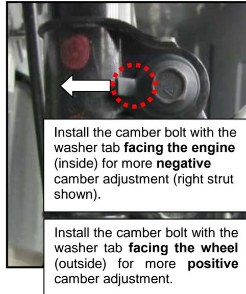
Install the camber bolt with the washer tab **facing the engine** (inside) for more **negative** camber adjustment (right strut shown).
