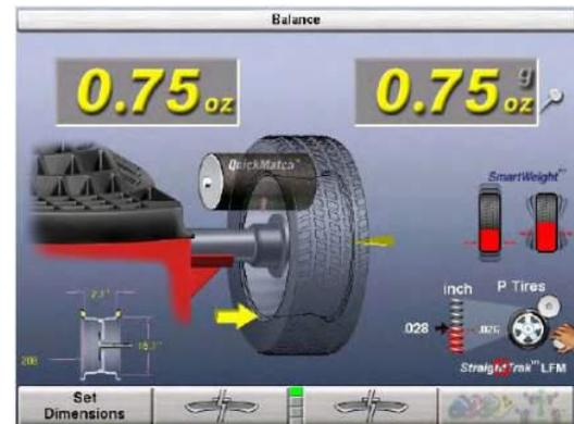
2. After balancing, press the tire tag button located at the bottom right of the screen to assign a number to that assembly. Label the assembly accordingly with a tag or chalk mark.
