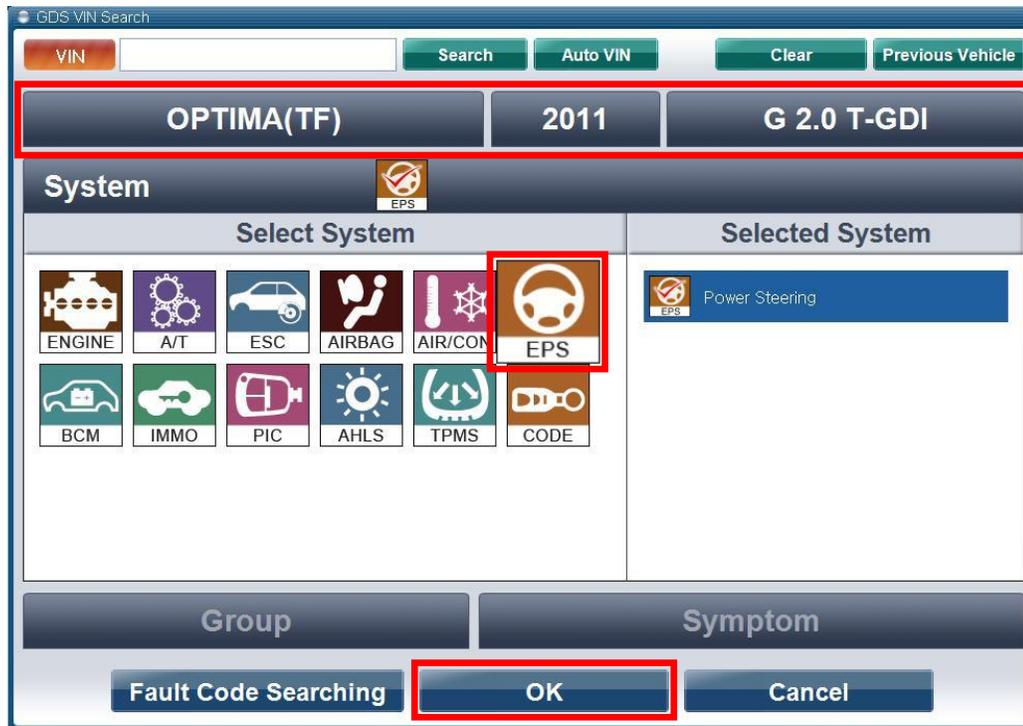
6. Enter the vehicle information by pressing the **VIN Auto Detect** button, entering the vehicle's VIN or selecting the vehicle model, model year, engine/fuel type and **EPS** as the system and then click **OK**.
