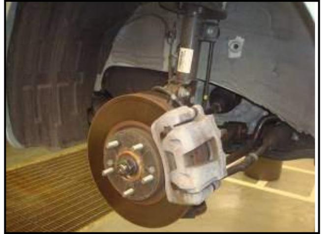
2. Remove upper strut-to-knuckle mounting nut and bolt.
