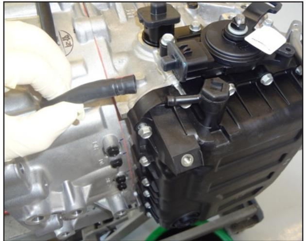
8. Remove the valve body cover. Detailed removal/installation steps vary depending on model. The valve body cover can be removed from all models listed in this TSB without removing the transaxle from the vehicle.
