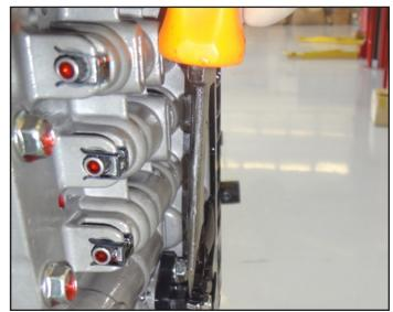
11. Remove the transaxle temperature sensor after removing the bolt. Replace with a new sensor and re-connect the harness to the sensor.
