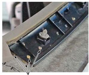
Use enough epoxy so that excess epoxy squeezes out of the holes and edges.
