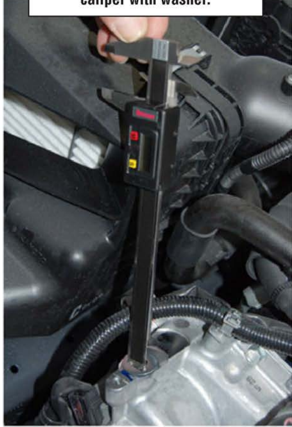
Measurement taken using digital caliper with washer.
