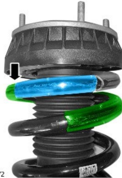
5. Correct installed condition.
