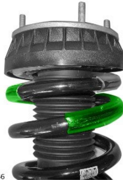
6. Install the rear right shock absorber / coil spring assembly (see TOPIx Workshop Manual, Section 204-02, reversing steps 1-5).
