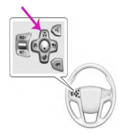
Press the follow distance gap button to select a follow distance gap (or time) setting for ACC of Far, Medium, or Near.
