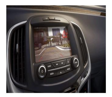
A warning triangle may display on the RVC screen to show where the Ultrasonic Rear Parking Assist (URPA) has detected an object. This triangle changes from amber to red and increases in size the closer the object.
