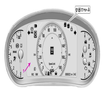
There is an interactive display area (1) in the **center** of the instrument cluster. The displays show the status of many vehicle systems. The controls for the DIC items and displays are on the right steering wheel control pad.
