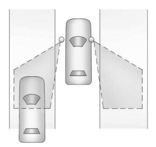
The SBZA sensors cover a detection zone from approximately the middle of the vehicle, one lane over from both sides of the vehicle, approximately 11 ft (3.5 m) and extends rearward approximately 16 ft (5 m). The height of the zone is approximately between 1.5 ft (0.5 m) and 6 ft (2 m) off the ground.
