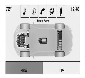
Engine Power - Engine is active with energy flowing to the wheels.
