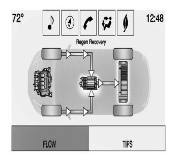
**Regen Recovery** - Power from the wheels returns to the battery during regenerative braking or coasting.
