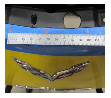
8. Measure 50 mm on both sides of the center point and mark with a paint pen creating a 100 mm application area.
