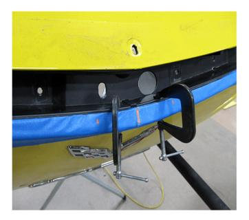
13. Clamp the lamp bracket the fascia as shown and allow the adhesive to cure per the manufacturers instructions. **Note:** Test fit the CHMSL to ensure the repositioned lamp covers the damaged paint edge on the fascia. If the paint damage is not covered by the lamp, repair the paint as required.
