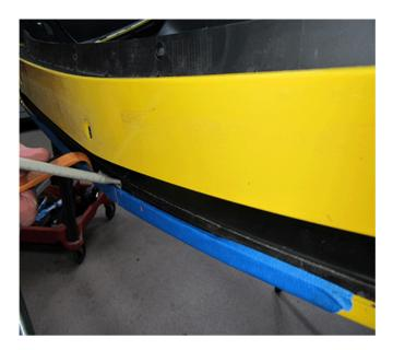
12. Apply a 10 mm bead of adhesive between the lamp bracket and the inner fascia as show.
