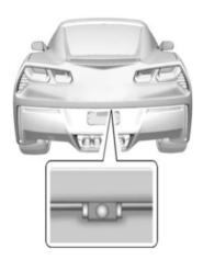
This vehicle has a rear vision camera (RVC) system. The RVC system can assist the driver when backing up by displaying a view of the area behind the vehicle. The RVC system has a guideline overlay that can help the driver align the vehicle when backing into a parking spot. The camera is mounted above the license plate in the position shown. The top of the license plate should be visible. **DO NOT** attempt to adjust or move the RVC camera.
