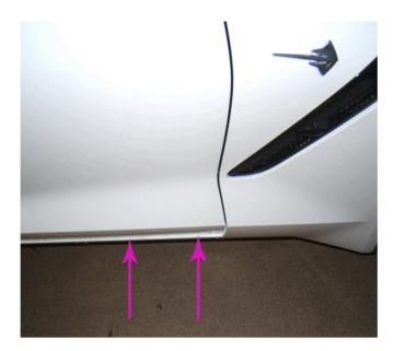
The front top of the rocker molding is designed to be outboard of the bottom of the front lower door by approximately 13 mm. This is a design feature and **does not** require adjustment.
