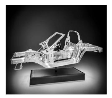
The 2014 Corvette Stingray utilizes an all-new aluminum frame structure that's lighter and stronger than the previous steel frame. The new aluminum frame structure is 57 percent stiffer and 99 pounds (45 kg) lighter than the steel frame used on the previous generation.
