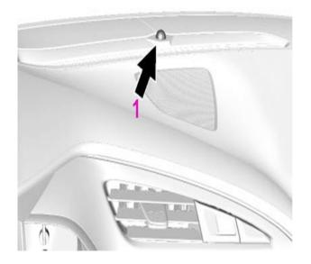
When the exterior lamp control is set to **AUTO** and it is dark enough outside, the headlamps and parking lamps turn **ON** automatically. There is an ambient light sensor (1) on top of the instrument panel. **DO NOT** cover the ambient light sensor (1), otherwise the headlamps will turn **ON** when they are not needed.
