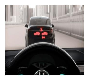
If ACC is engaged, driver action may be required when ACC cannot apply sufficient braking because of approaching a vehicle too rapidly. When this occurs, the flashing red collision alert symbol will display on the Head-Up Display (HUD). Either eight beeps will sound from the front, or both sides of the Safety Alert Seat will pulse five times.
