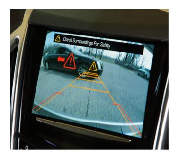
Displayed images may be farther or closer than they appear. The area displayed is limited and objects that are close to either corner of the bumper or under the bumper do not display. A warning triangle may display on the RVC screen to show where the RCTA has detected an object. This triangle changes from amber to red and increases in size the closer the object.
