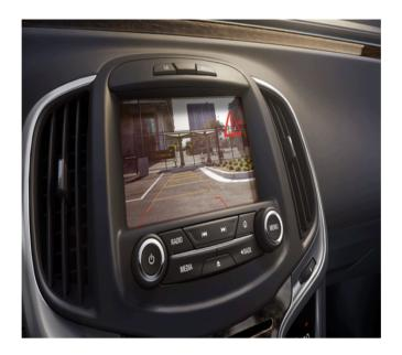
If equipped, the Rear Vision Camera (RVC) displays a view of the area behind the vehicle, on the center stack display, when the vehicle is shifted into R (Reverse). Some models may also have the Rear Cross Traffic Alert (RCTA) feature which will also display a triangle with an arrow on the RVC screen to warn of traffic coming from either direction when backing.
