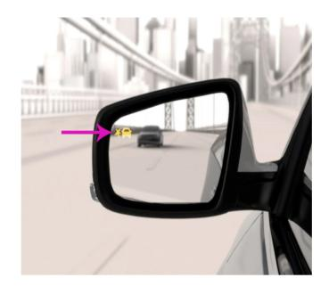
The LCA warning symbol will illuminate in the corresponding outside side mirror and will **FLASH** if the turn signal is **ON**. An illuminated or flashing LCA symbol indicates it may be unsafe to change lanes.
