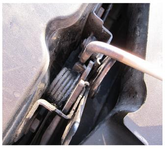
3. Rotate the release tool counterclockwise to push release lever.
