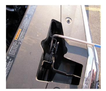
2. Turn end down into the center of the latch.
