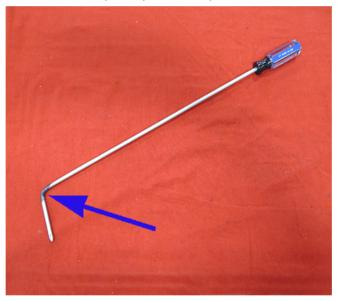
3. Clamp the screwdriver in a vise and create a 90° bend as shown.
