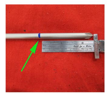
2. Measure and mark the screwdriver 63 mm (2.5 in.) from the tip as shown.
