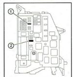
1 Install Short Pin Here 2 Remove This Short Pin
