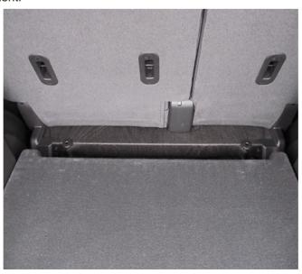
Starting with 2014 vehicle production, the floor filler trim panel was removed to increase rear stowage area. The seat/floor interface will now look like the example shown in the graphic above.
