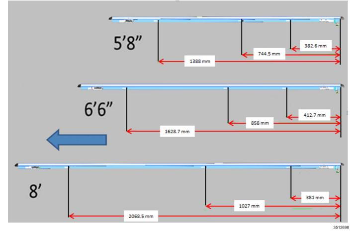
The image above shows the correct positioning for all clamps, depending on the pickup box length. Use the position dimensions and the steps below to install the clamps in the correct positions.
