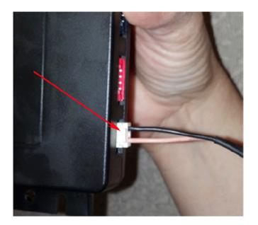
Incorrect Power and Ground wires
