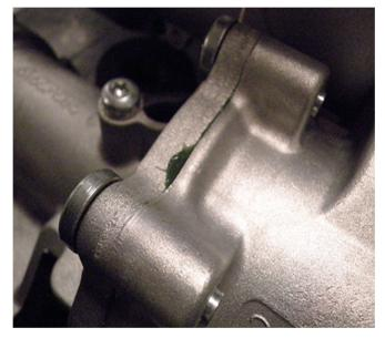
The graphic below shows a specific area where Loctite is used. The excess cured Loctite should also not be mistaken for an oil leak.
