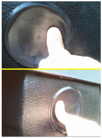
3. Continue pushing/seating the plug around both sides of the perimeter, from top to bottom.
