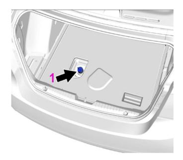
In the rear compartment of the vehicle, under the load floor is the DEF tank (1). The capacity of the tank is 4.9 gallons (18.5 L). This is enough DEF to provide a range of at least 10,000 miles (16,000 km) of driving between refills. The system is also designed for servicing to coincide with oil changes, for greater convenience.
