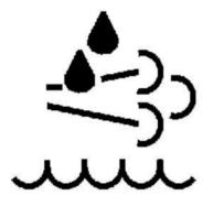
The **DIESEL EXHAUST FLUID WARNING LIGHT** will turn **ON**, a DIC Message will display and a chime will also come **ON**, if there is an issue with the Diesel Exhaust Fluid. If the fluid issue is not corrected, the light will continue to flash when the vehicle is started. While driving, the vehicle's speed may be limited.
